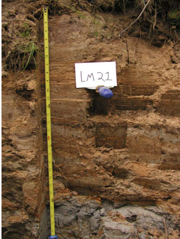
Figure 3.7: Outcrop at ID 168 illustrating facies change to silty sand overlying gray clay.
